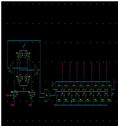
Fig 3: Architecture of the complete low power 8-bit SAR ADC
