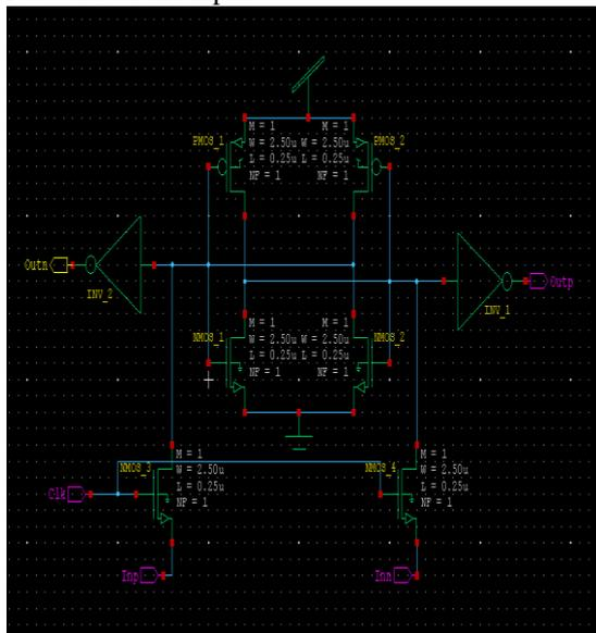
Fig 1: Schematic of Proposed Double Edge Triggered Comparator
