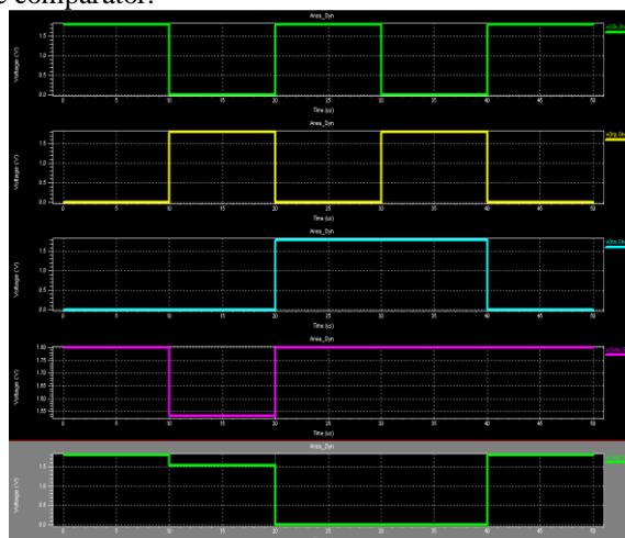
Fig 2: Simulation Result of Proposed Comparator
